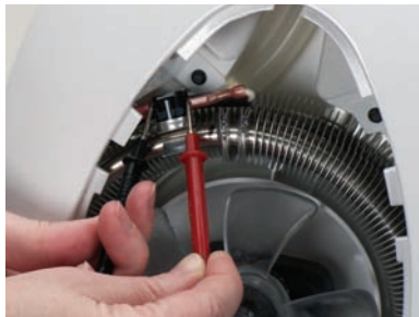
Figure M – testing condensing coil thermostat
