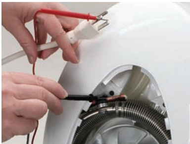
Figure L – testing fan motor
