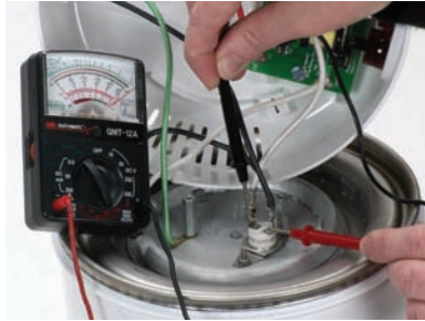
Figure J – testing thermostat
